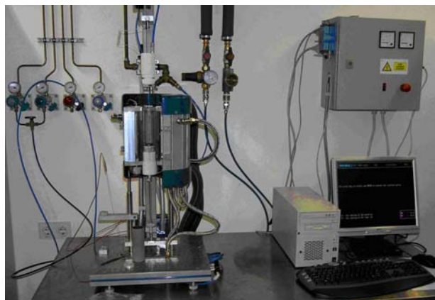
Apparatus for expansion measurement on foamable metallic precursors
