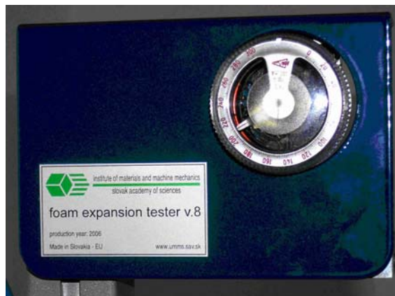
Apparatus for expansion measurement on foamable metallic precursors
